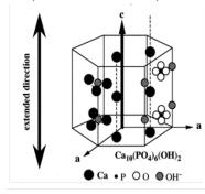
Figure 01- Crystal structure of the Hydroxyapatite
