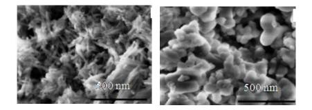
Figure 02. SEM images of (a) Needle-like HA nanoparticles (b) spherical shape HA nanoparticles.
